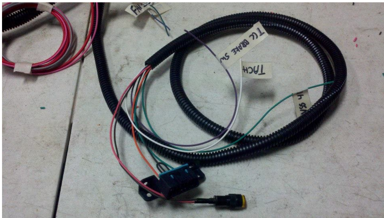
OBD2 port, check engine light, tach, VSS, and TCC brake switch wires.
